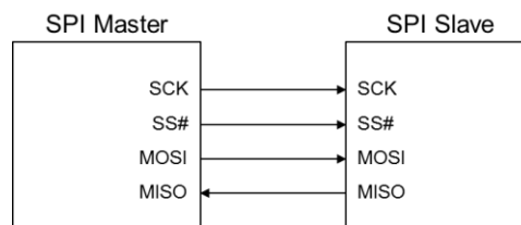
Figure 1. SPI Master and SPI Slave Connection
