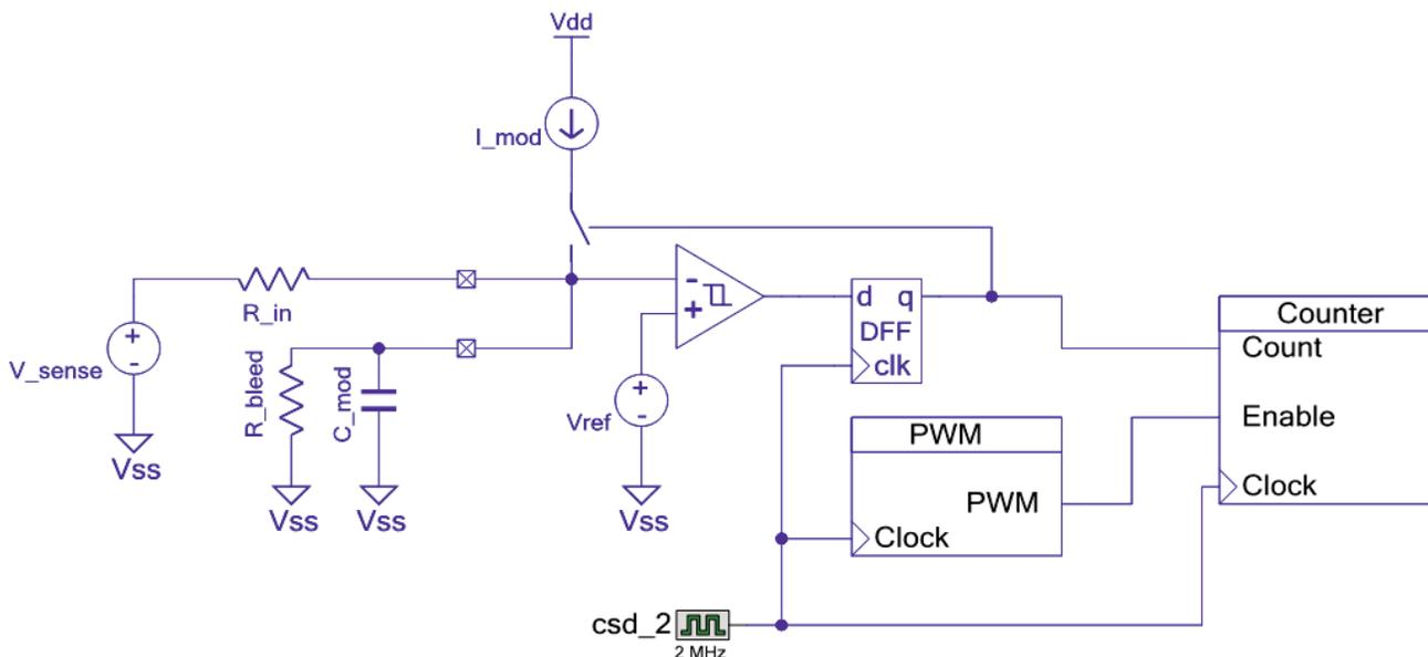
The ratio of on time to off time is measured by the counter over a fixed period of time. The ratio of on time to off time relative to  $I_{mod}$  represents the average current pulled out of  $C_{mod}$  by  $R_{bleed}$  and the input.
