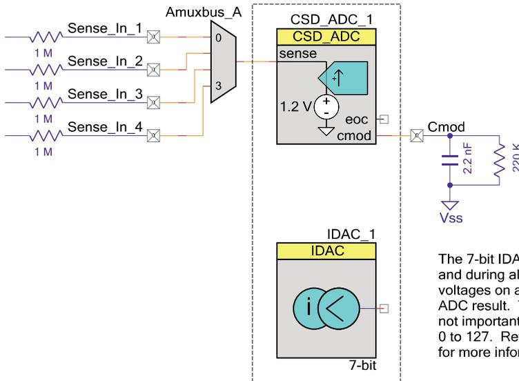
The 7-bit IDAC must be enabled prior to, and during all ADC conversions to prevent voltages on amuxbus B from affecting the ADC result. The output current of the IDAC is not important and can be anything from 0 to 127. Refer to the CSD\_ADC datasheet for more information.
