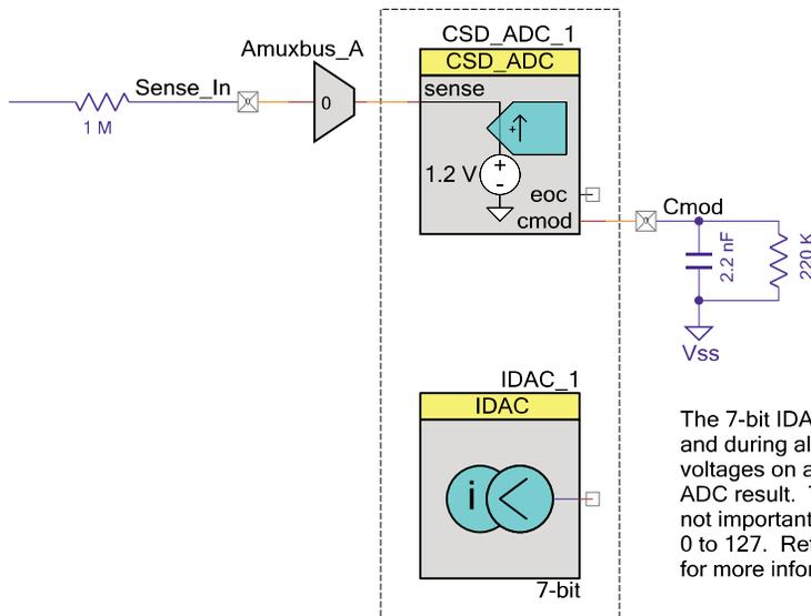
The 7-bit IDAC must be enabled prior to, and during all ADC conversions to prevent voltages on amuxbus B from affecting the ADC result. The output current of the IDAC is not important and can be anything from 0 to 127. Refer to the CSD\_ADC datasheet for more information.
