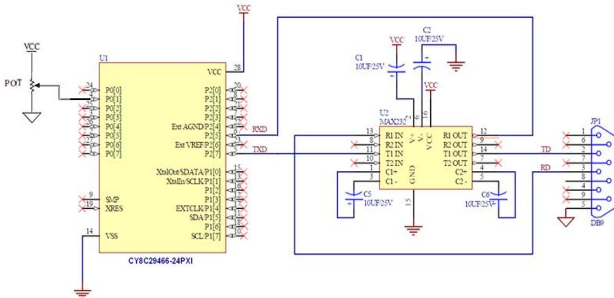
MAX232, an RS232 transceiver, is used to translate the +/-10V RS232 signals to transistor-transistor logic (TTL) level signals of the PSoC.
