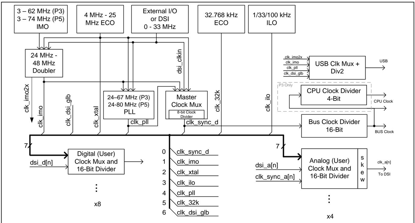
Figure 1 PSoC 3 and PSoC 5LP Clock Overview Diagram
