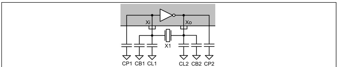
**Figure 4 ECO Circuit with Parasitic Capacitances Shown**
