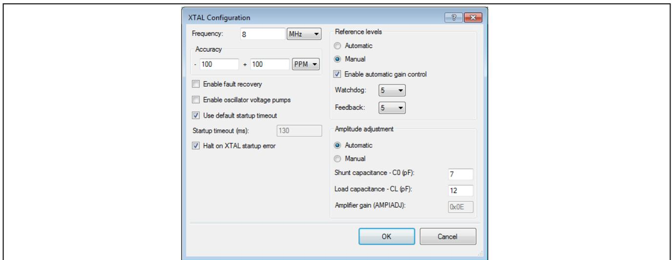
**Figure 7 Example PSoC Creator MHz ECO Configuration Dialog**
