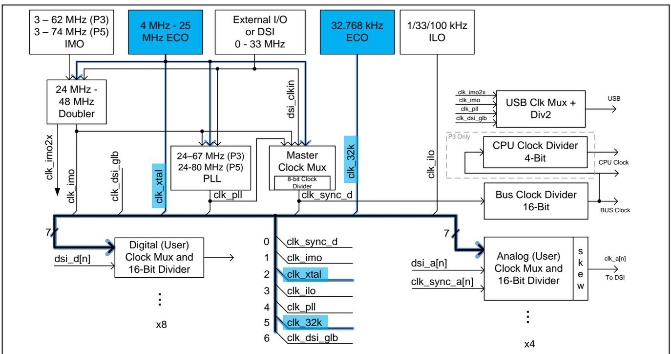
**Figure 5 PSoC 3 and PSoC 5LP Clocking Tree with ECOs Highlighted**
