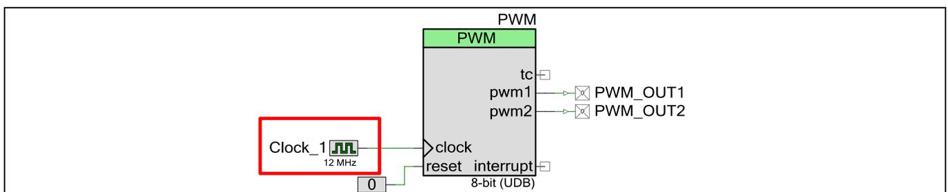
Figure 13 Using Clocks in PSoC Creator
