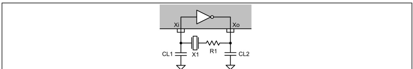
**Figure 8 ECO Circuit for Negative Resistance Tests**
