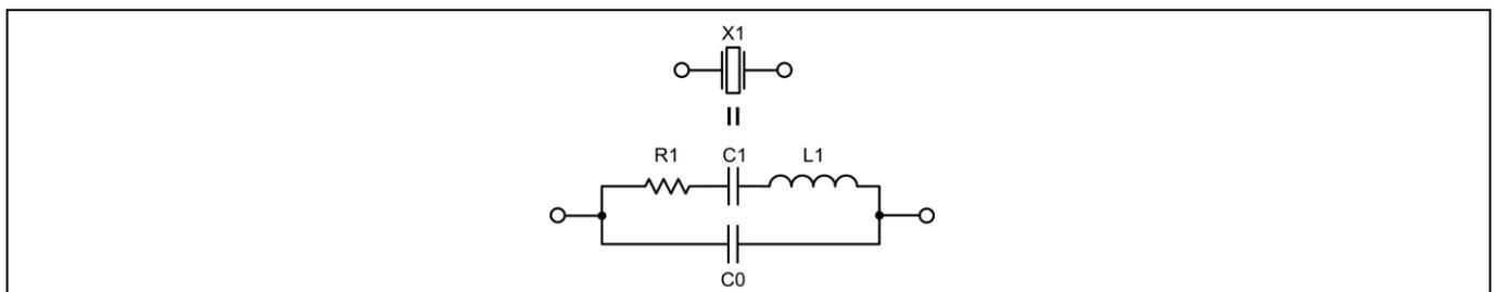
Figure 10 Resonator Equivalent Circuit
