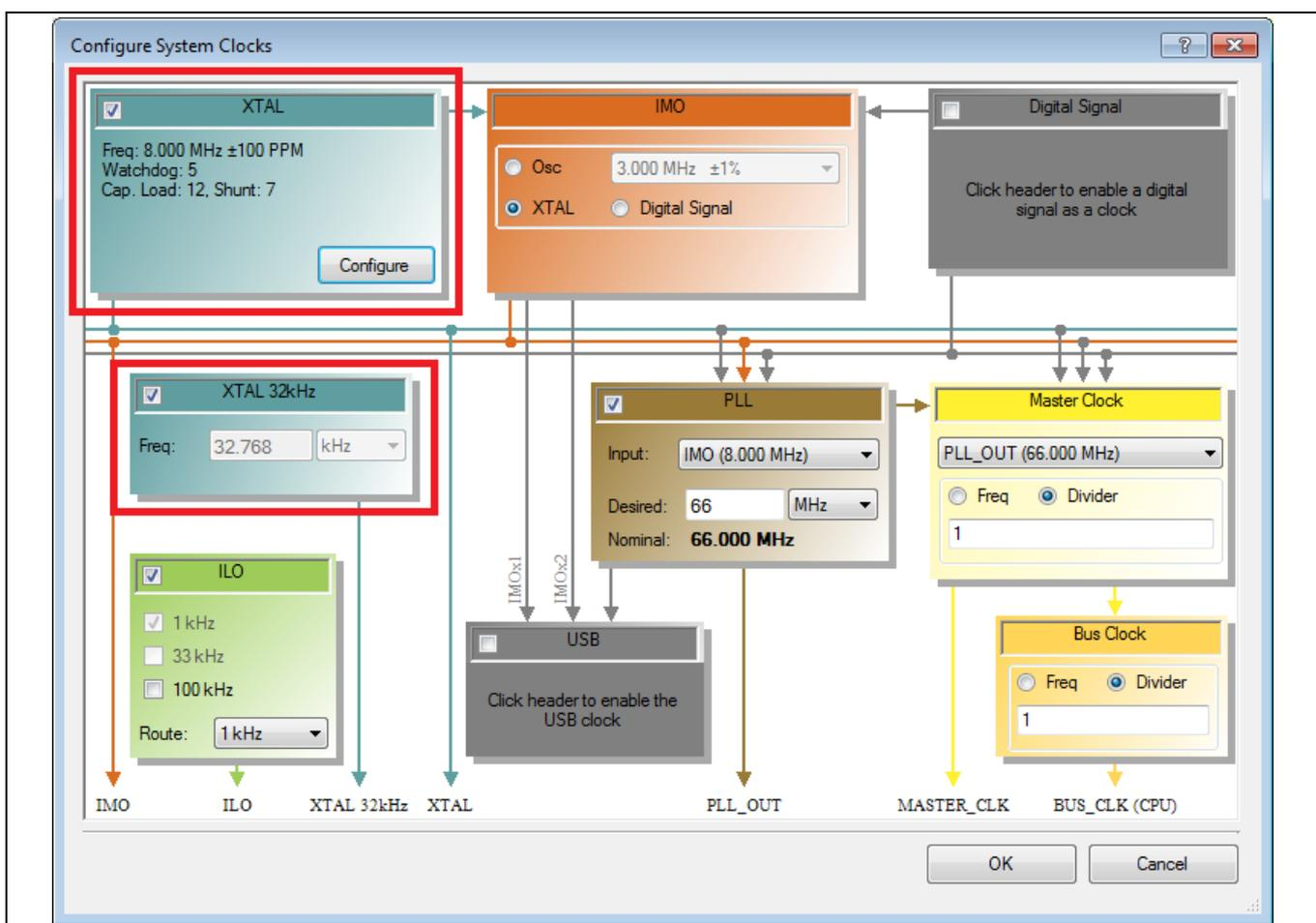
Figure 6 Example PSoC Creator Configure System Clocks Dialog with ECOs Highlighted
