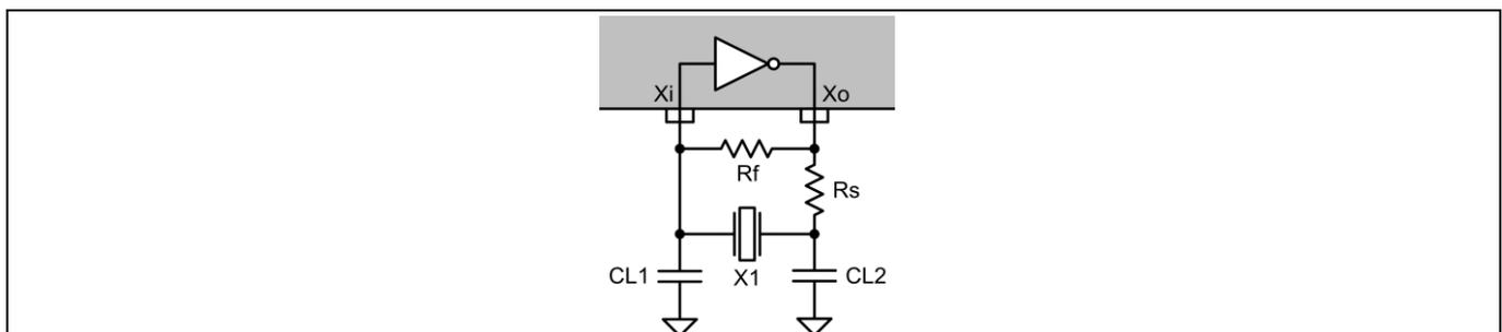
**Figure 11 Pierce Oscillator Topology with Series and Feedback Resistors**
