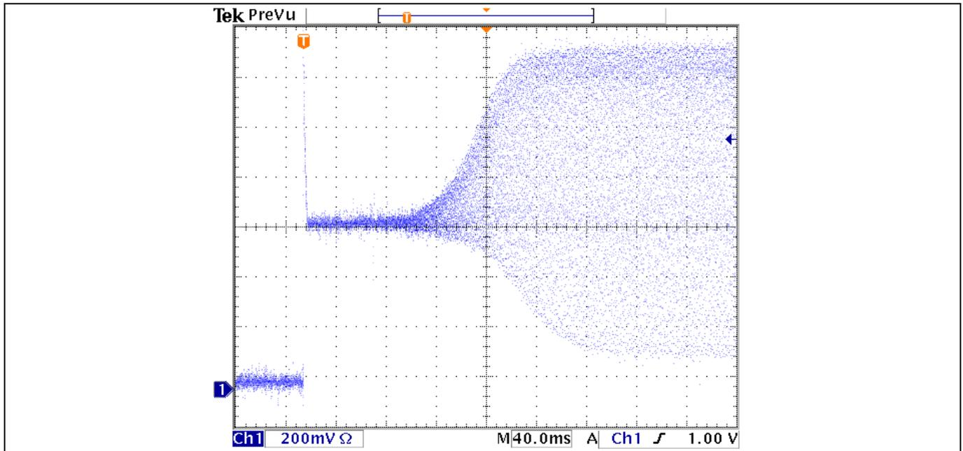
Figure 12 32-kHz ECO Startup Behavior
