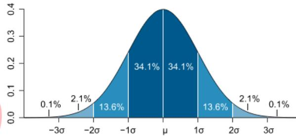
Statistical analysis obtained from a set of random boards helps to predict the variation of data that exists in the entire set of boards. If the average of the data set is denoted by  $\mu$  and standard deviation by  $\sigma$ , then basic theorem says that 68.2 percent of data falls between the  $\mu - \sigma$  and  $\mu + \sigma$ . Similarly, 95.4 percent of data is between  $\mu - (2\sigma)$  and  $\mu + (2\sigma)$  and so on.
