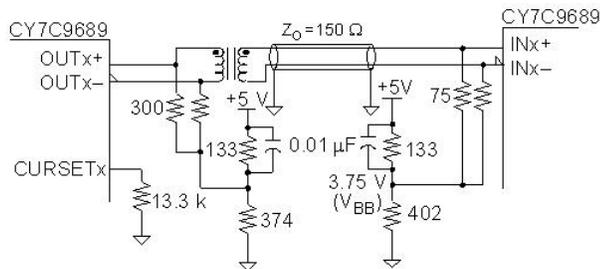
The transformer is similar to a capacitor in that it also has passband characteristics, limiting both low- and high-frequency operation. Proper selection of a coupling transformer allows passing of the frequencies necessary for HOTLink serial communications. A schematic detailing a transformer coupled interface is shown in Figure 10.
