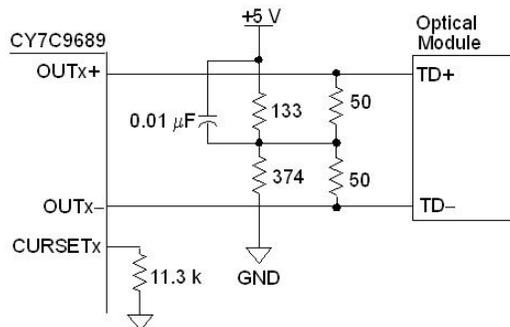
Figure 6. CY7C9689 Transmitter to ECL Optical Module
