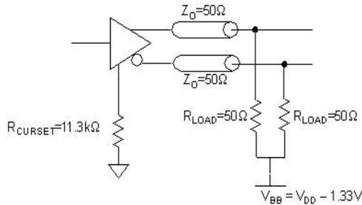
In Equation 1,  $V_{OPP}$  is the difference in voltage levels at one output of the differential driver when that output is driving HIGH and LOW, and  $Z_{LOAD}$  is that load seen by the one output when it is sourcing and sinking current. With known load impedance and a desired signal swing, it is possible to calculate the value of the associated CURSETA or CURSETB resistor that sets this current.
