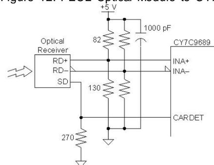
Figure 13. ECL Optical Module to CY7C9689
