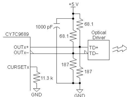
To reduce the impact of impedance mismatches, stub effects, and reflections, the signal-trace routing from the CY7C9689 serial output to the optical module data inputs should be kept as short as possible. To maintain proper balance in the transmission line, the length of the two traces must remain equal (both physically and electrically), such that minimal skew exists between the differential signals.
