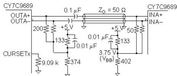
For either type of DC-coupled transmission line (dual unbalanced or single balanced), either the dual Thévenin or the H-bias termination may be used. For the lowest power dissipation, H-bias should be used.
