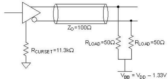
Figure 4. CY7C9689 Transmitter to PECL Optical Module: Thévenin Termination
