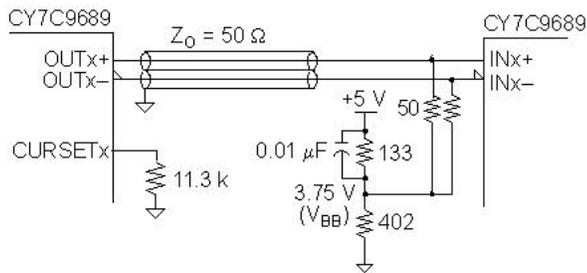
Figure 9. Capacitive-Coupled, Copper Interface
