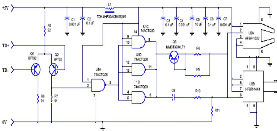
Figure 3. +5 V ECL (PECL) Compatible 160 MBd Fiber-Optic Receiver
