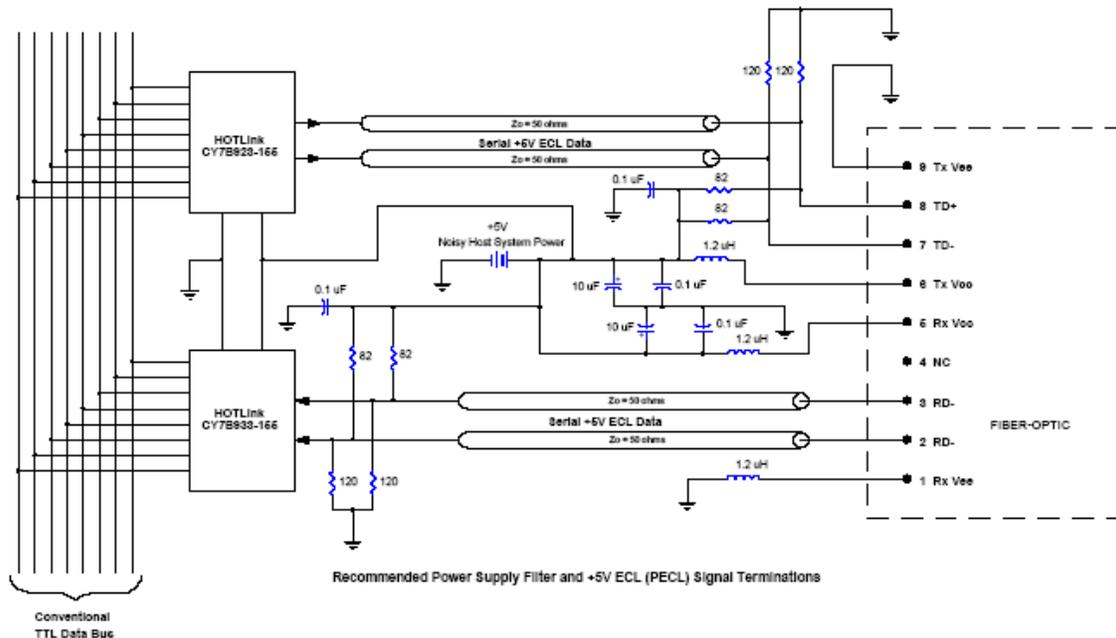
When used with HOTLink, the power supply filter and terminations shown in [Figure 6](#) are recommended. In this environment, the transceiver in [Figure 4](#) has been proven to provide excellent performance. The capacitor values are chosen based on series resonance considerations as discussed in the Cypress application note [AN1032 - Using Decoupling Capacitors](#).
