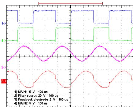
Figure 18. 2-Pin Oscillator Parallel Resonance Mode
