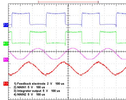
Figure 15. 3-Pin Oscillator Waveforms
