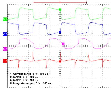
Figure 16. 3-Pin Oscillator Waveforms
