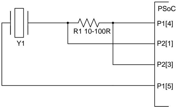
When the resonator's current reaches zero and the voltage polarity reverses, the instrumentation amplifier changes the output signal sign, which is detected by switching the switched capacitor block's zero-crossing comparator. The comparator changes the voltage polarity at the piezoelectric plane electrodes, which causes the current to increase through the resonator, thus matching the phase balance rule.
