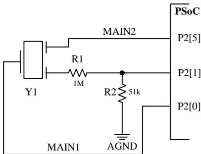
The feedback electrode output voltage is greater than the typical power supply level. The resistors  $R_1$  and  $R_2$  combined with the switched capacitor block input stage impedance form the voltage divider and limit the PSoc device's input pin current. Note that the resistor  $R_2$  does not have to be used because the switched capacitor block input acts as a resistor connected to the PSoc device's AGND. The rest of the oscillator circuit is implemented inside the PSoc device.
