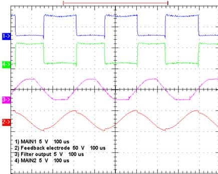
Figure 17. 3-Pin Oscillator Waveforms
