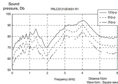
As seen from [Figure 5](#), to achieve the maximum sound pressure level, the excitation frequency should equal the resonant frequency. This frequency depends on:
