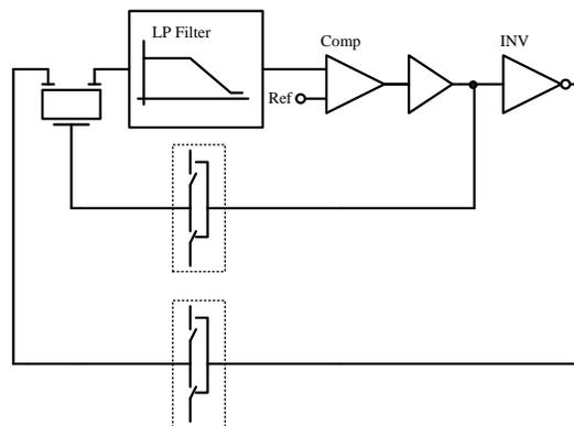
The buzzer's feedback output electrode signal through a matching circuit is passed to the second order LPF; and the amplified and phase-delayed signals are passed to the comparator. The digital comparator signal is routed via inverting/non-inverting buffers to the buzzer, closing the feedback loop. The oscillator operates at series resonance.
