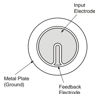
Buzzers with 3 pins (see [Figure 1](#)) are manufactured for resonance oscillators specifically; the feedback signal can be used for switching excitation voltage. There are resonators without the separate feedback electrode; they are called 2-pin resonators.
