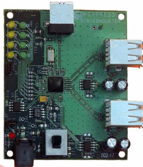
Cypress offers the TetraHub reference designs as an evaluation platform for developers wishing to integrate a USB 2.0 hub into their application. The designs are examples of a self-powered, 4-port USB 2.0 hub or a bus powered, 2-port hub. The kits includes the hub evaluation board, USB cable, power supply, schematics, bill of material, PCB Gerber files, and other documentation.
