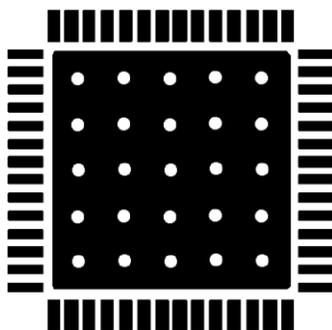
The signal ground plane provides the major area for thermal dissipation. The CY4602 uses the large internal layer of the PCB devoted to signal ground. This is a fairly large board intended for demonstration and evaluation of the CY7C65640A component.
