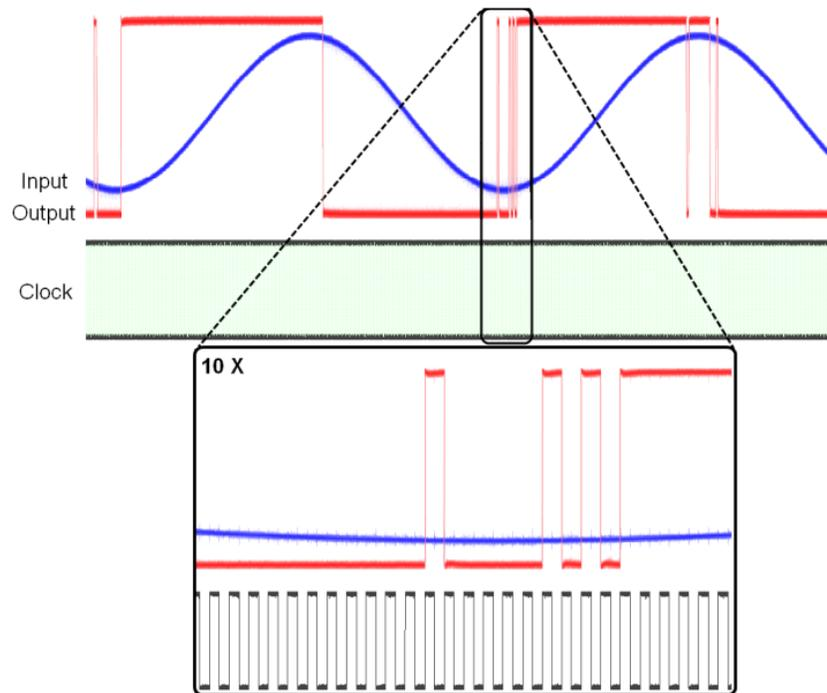
Figure 4 shows the effect when the clock speed is set too low. Notice that the output should be high during the positive slope; the output is severely delayed from the input waveform. Some peaks may be missed altogether. In this case, the clock rate is 2.5x the frequency of the 1 V peak-to-peak input sine waves; the input is sampled only two or three times per cycle.
