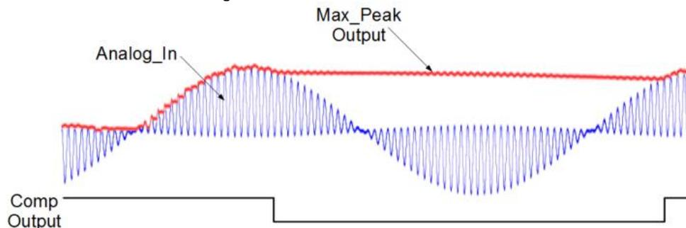
The output of the sample and hold will decay over time. Refer to the Mixer [datasheet](#) for specifications on this droop voltage. The output of the sample and hold will droop towards the supplied reference voltage for the sample and hold component. By changing your reference to  $V_{DDA}$  and inverting the comparator polarity, a minimum peak detector can be created.
