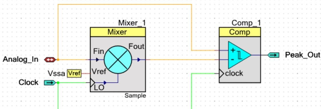
A down mixer is used as a sample and hold whose output is fed to a comparator and compared to the original input signal. The output of the sample and hold is held on the falling edge of the sample (LO) clock. The comparator is clocked on the rising edge of the sample clock which creates a half clock cycle delay between the two signals at the comparator. This ensures the sampled signal is stable and appropriately delayed from the input signal. This concept is illustrated in Figure 2.
