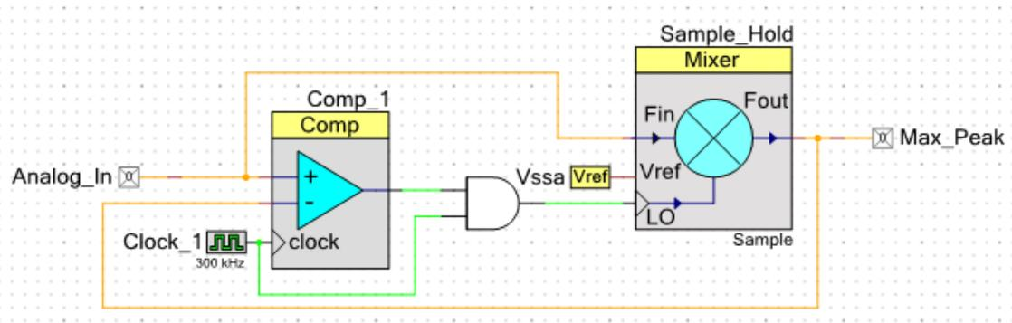
With this configuration, the sample and hold component is clocked only if the analog input is greater than the last maximum value held at the output. When the analog input is greater than the last held value, the comparator output asserts and the sample and hold is clocked to update the output to a new maximum value. Comparator hysteresis is not needed for this configuration. Figure 12 shows the output waveform for this peak detector.
