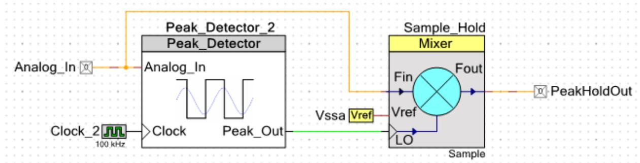
At every peak from the peak detector component, the original input waveform is sampled by another sample and hold component. Because the output of the sample and hold is held on the falling edge of the LO input clock, each peak is held at the output until the next peak is detected. To create a negative peak and hold, simply invert the output polarity of the peak detector component. The output of the peak and hold circuit is shown in Figure 10.
