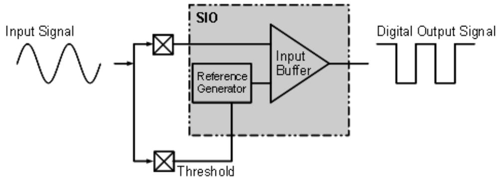
Figure 8 shows the expected waveforms for the SIO peak detector circuit. The threshold input is delayed by approximately 200 ns, which allows the differential input buffer (acting as a comparator) to detect the peaks in the input waveform.
