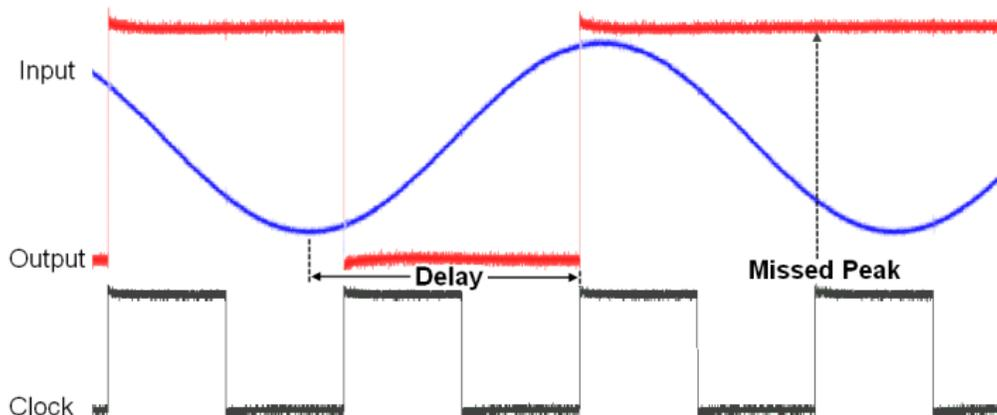
Figure 5 shows the output when the correct clock is selected. There is very little delay between the input peaks and the output; there are no erroneous triggers or missed peaks. In this case, the clock rate is 50x the frequency of the 1-V peak-to-peak input sine wave.
