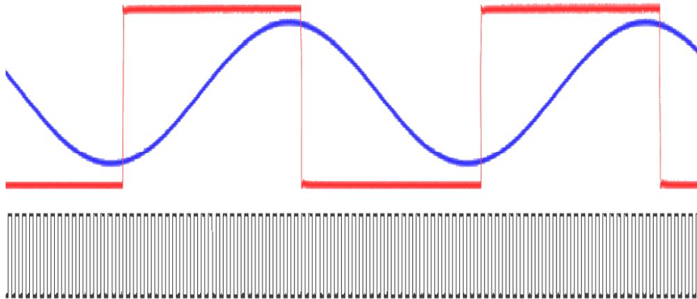
The appropriate clock speed differs for each application, depending on the frequency and noise characteristics of the input waveform.
