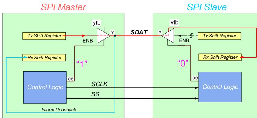
**Figure 2. SPI Bidirectional Mode (data transmission from Slave to Master)**
