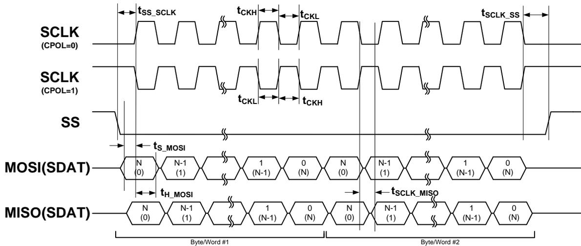
**Figure 7. Mode CPHA = 1 Timing Diagram**
