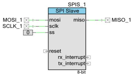
**Figure 4. 3-wire (Bidirectional) Interfacing Schematic Macro**
