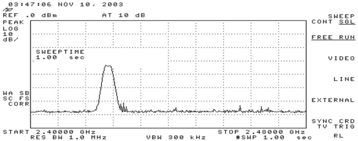
Figure 12 shows a DSSS cordless phone signal and a WirelessUSB LP/LPstar signal that slightly overlap, but not enough to cause interference. Both systems function normally without any loss of quality.
