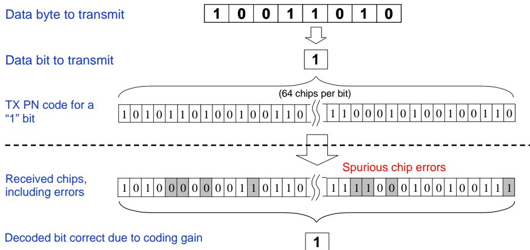
If the correlator error threshold is exceeded, the received data bit is not corrupted but erased. There is a negligible probability of data being corrupted rather than erased, because this would require interference to corrupt the majority of chips in such a way that the incoming data stream correlated with the PN code corresponding to the
