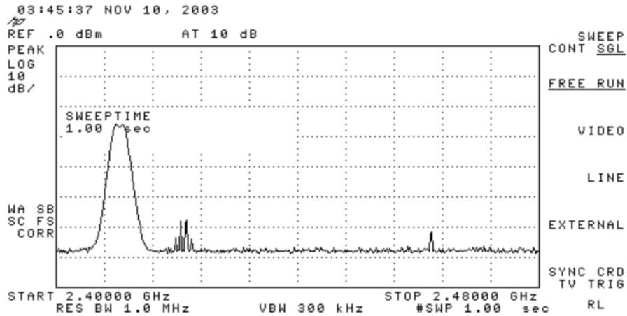
Figure 11 shows overlapping DSSS cordless phone and WirelessUSB LP/LPstar signals. In this situation the WirelessUSB LP/LPstar traffic is corrupted and the corrupt packet threshold monitor causes the WirelessUSB LP/LPstar devices to change channels and move away
