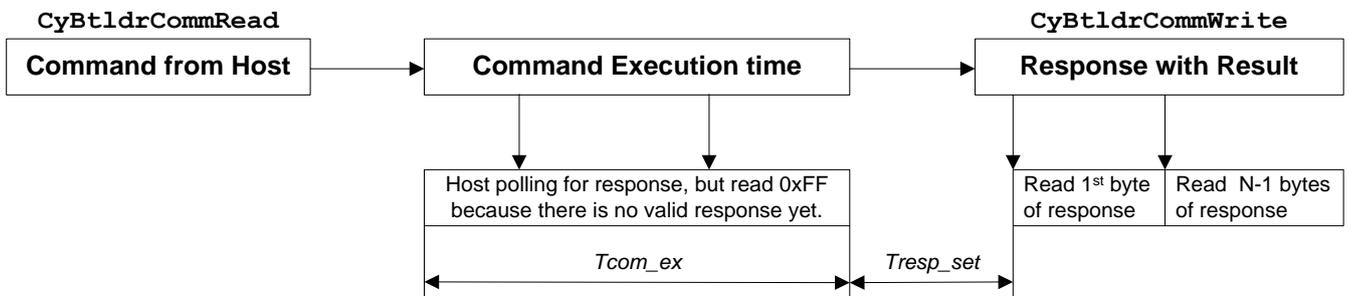
The host must execute polling by reading one byte; reading more bytes could corrupt the response. For example, in the case of 0xFF 0x01 0x03 (two bytes of response were read, instead of one), the next read of the full response returns two invalid bytes, because these bytes were already read (0x01 and 0x03).
