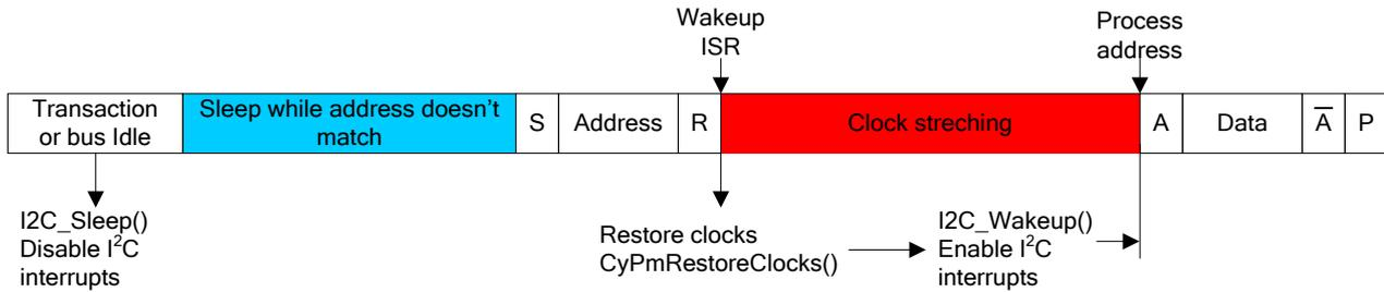
**Bootloader Protocol Interaction with I<sup>2</sup>C Communication Component**
