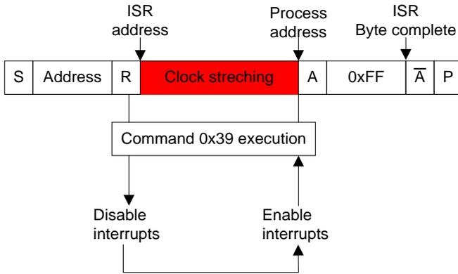
**How to avoid clock stretching:** To avoid clock stretching, measure the Command Program Row (0x39) execution time ( $T_{com\_ex}$ ) according to the system settings (CPU speed, compiler, compiler optimization level). The host must ask for a response after this time.
