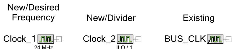
Clock components configured as "New" consume clock resources in the device and have APIs generated for them. Clock components configured as "Existing" to a system or design-wide clock do not consume any physical resources on the device and no APIs are generated for them. Instead, they use the selected system or design-wide clock.
