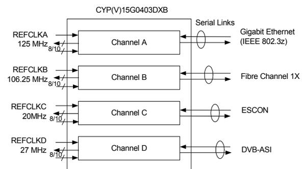
Figure 2. Example Of CYP15G0403DXB Transporting Data At Same Data Rate But Different Sources
