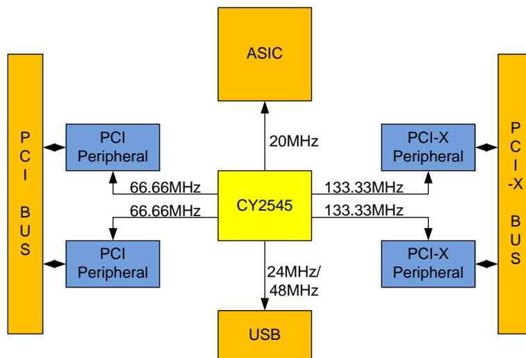
Two 133.33MHz and 66.66MHz clocks are edge aligned.
