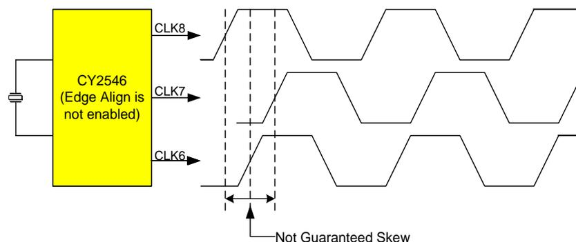
Alignment indicates basic phase alignment. The output-to-output skew is not zero, and a maximum skew can be as low as 200 ps between certain outputs (outputs from same PLL) measured at the output pins of the device.
