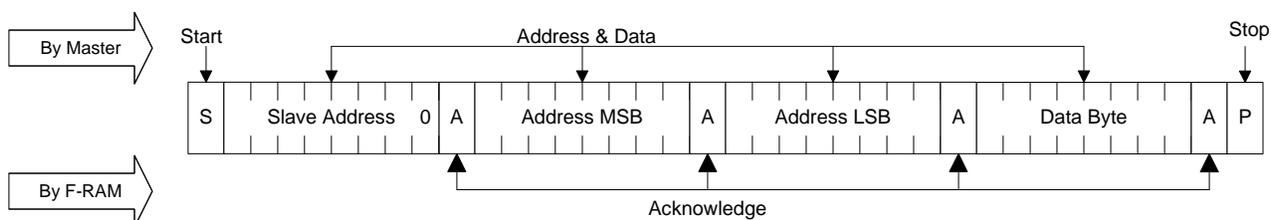
Figure 8. Multi-Byte Write
