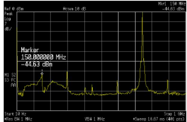
Figure 19. Channel A with Aggressor Channel C Sweeping Across the Operating Range
