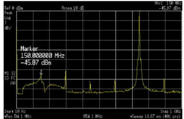
Figure 20. Channel A with Aggressor Channel D Sweeping Across the Operating Range
