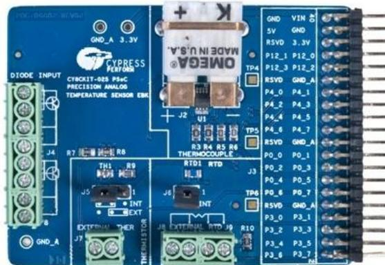
Figure 10. Thermocouple Section of the EBK
