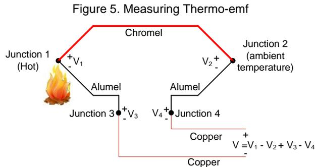
The input (copper) leads of the ADC form two more junctions (thermocouples) (copper-alumel) adding two more voltages,  $V_3$  and  $V_4$  to the equation.  $V_3$  and  $V_4$  are in opposite directions and they will have the same magnitude as long as both junctions are at the same temperature. Hence, we need to ensure that the two inputs into the ADC are at the same temperature so that the thermo-emf remains unchanged.
