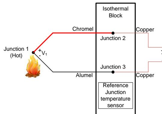
Measuring temperature using a practical thermocouple involves the following steps:
