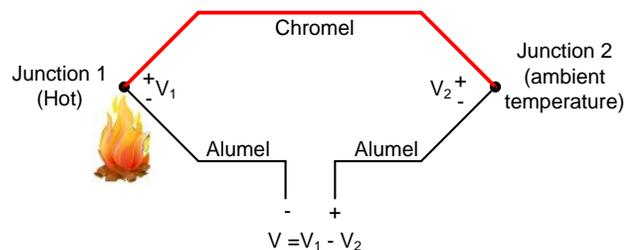
If the temperature of the cold junction is known, the voltage  $V_2$  can be calculated from NIST tables or polynomials. Therefore, in cases where the cold junction is not at  $0^\circ\text{C}$ , the cold junction temperature must be measured and the thermo-emf corresponding to that temperature must be added to the thermocouple voltage. This procedure is called cold junction compensation.
