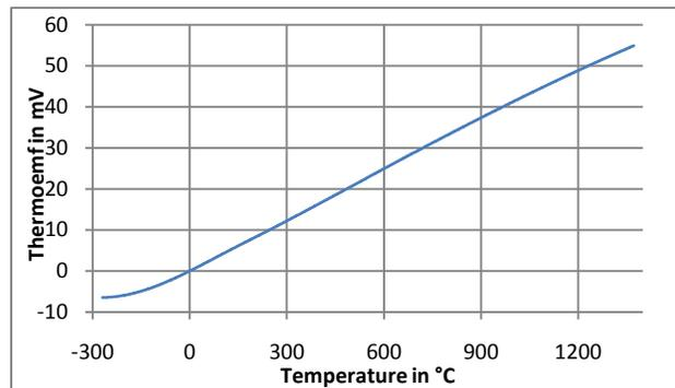
The sensitivity of a K-type thermocouple can be found from the NIST table and is approximately  $40 \mu\text{V}/^\circ\text{C}$  for temperatures  $> -100^\circ\text{C}$ . The NIST tables and coefficients can be found [here](#).
