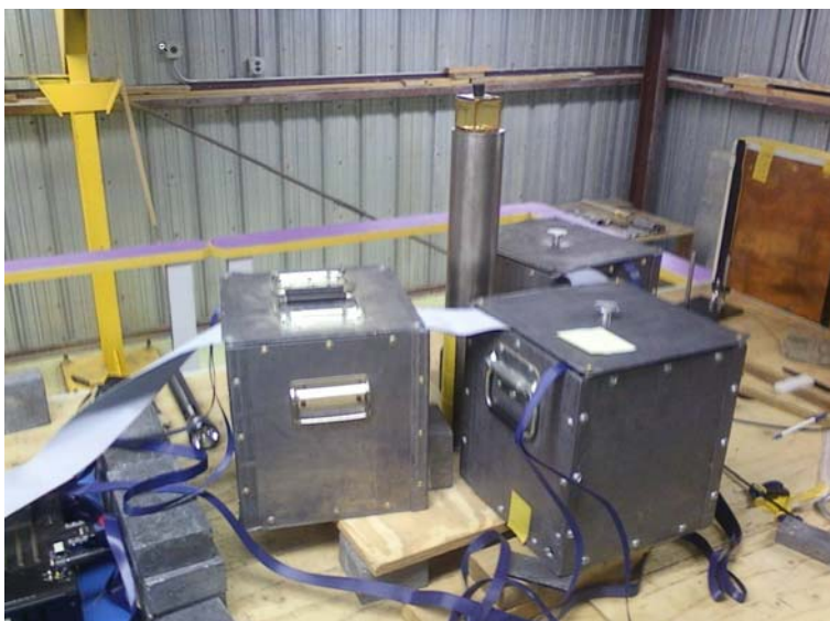
Figure 5. RLAT Devices being Irradiated in Lead/Aluminum Boxes at Co60 Facility
