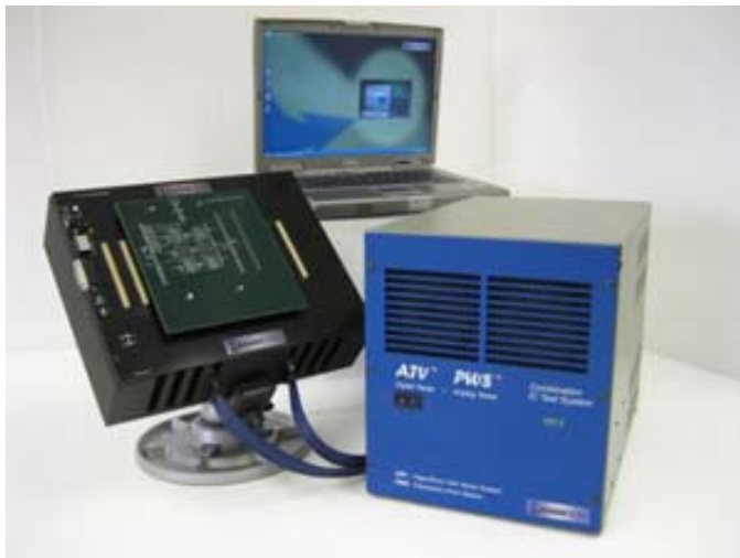
Figure 4. ATV Test System used for TID Testing
