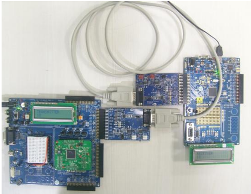
Figure 21. CAN Physical Connections
