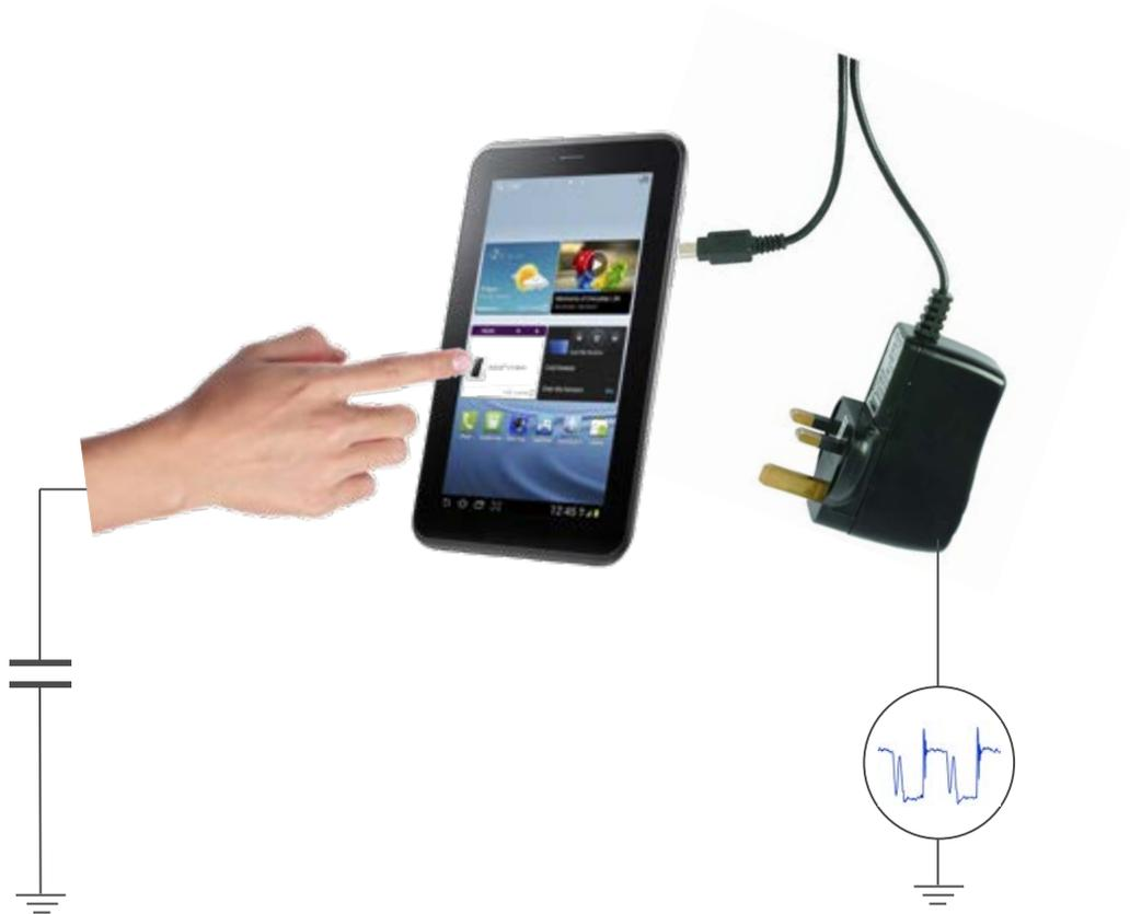
**Figure 2. Coupling of the common-mode noise through the touchscreen**
