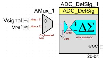
$$\text{Equation 4 } V_{\text{out1}} = (V_{\text{signal}(T1)} - V_{\text{gnd}(T1)}) + V_{\text{offset}(T1)} + V_{\text{noise}(T1)}$$
