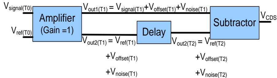
Based on Figure 1, the signals at the input of the subtractor are as follows:
