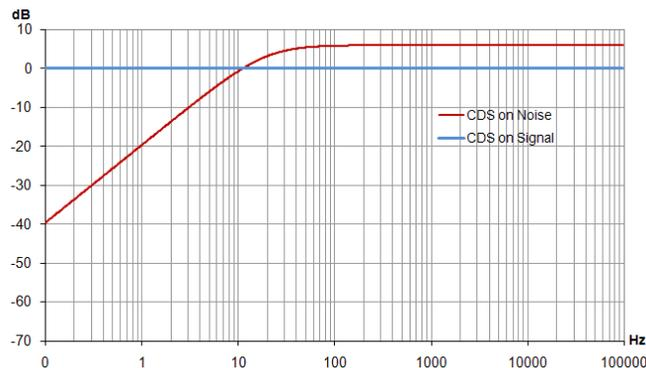
When high-frequency noise has to be eliminated along with low-frequency noise, CDS must be followed by an infinite impulse response (IIR) filter.
