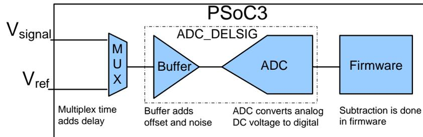
The ADC converts the input and reference signals into the digital domain. These values are then accessed and subtracted in firmware.
