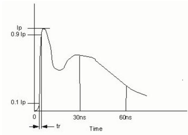
The peak current value is 30 Amperes,  $t_r$  is about 1 nanosecond, current at 30ns is about 16 Amperes, and the current at 60ns is about 8 Amperes (from ref. 9) for a range of current.
