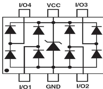
The diodes provide clamping to the rails as well as reverse breakdown protection. They are not intended to operate in the forward current mode except transiently.
