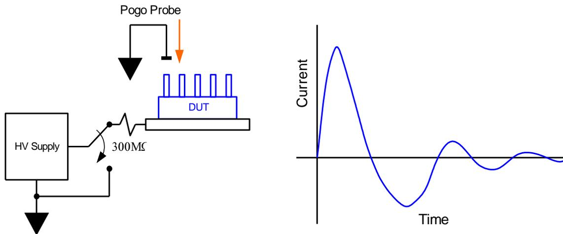
The device is charged electrostatically through a dielectric then connected to ground. A probe is used to record the current waveform through the discharge path.
