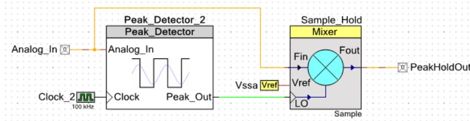
Figure 8. Peak and Hold Schematic
