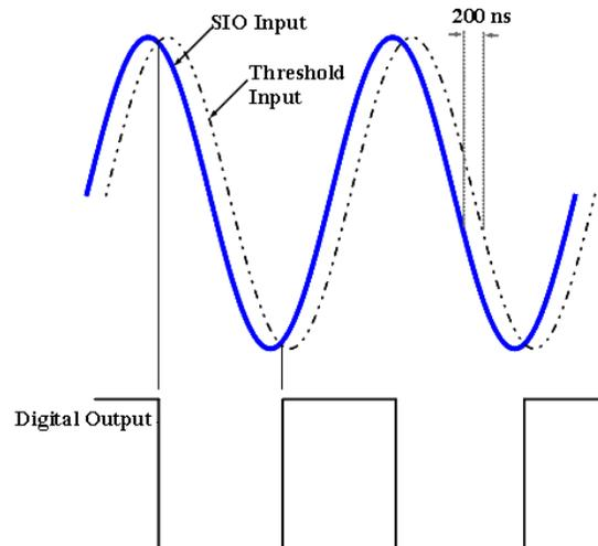
**Figure 7. SIO Peak Detector Waveform**
