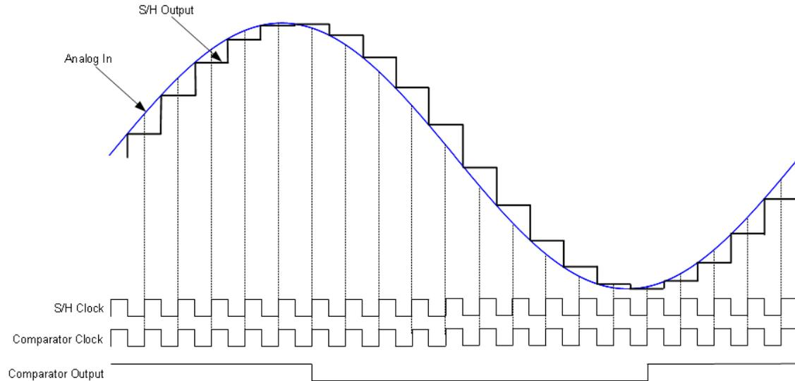
**Figure 1. Sample and Hold Peak Detection Waveform**
