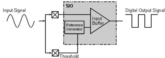
**Figure 6. SIO Peak Detector Block Diagram**
