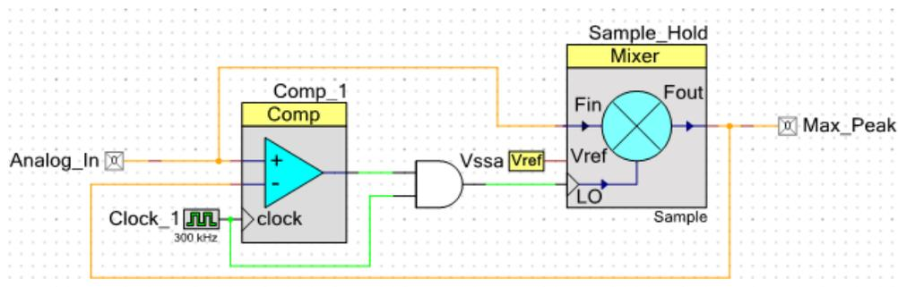
Figure 10. Maximum Peak Detector Schematic
