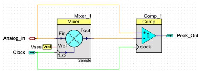
Figure 1. Peak Detector with Sample and Hold
