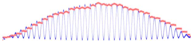
Figure 9. Peak and Hold Waveform
