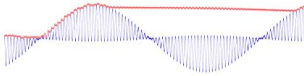
**Figure 11. Maximum Peak and Hold Waveform**
