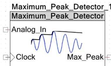
**Figure 12. Maximum Peak Detector Component Symbol**
