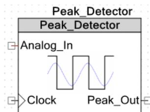
Figure 5. Sample and Hold Peak Detection Component
