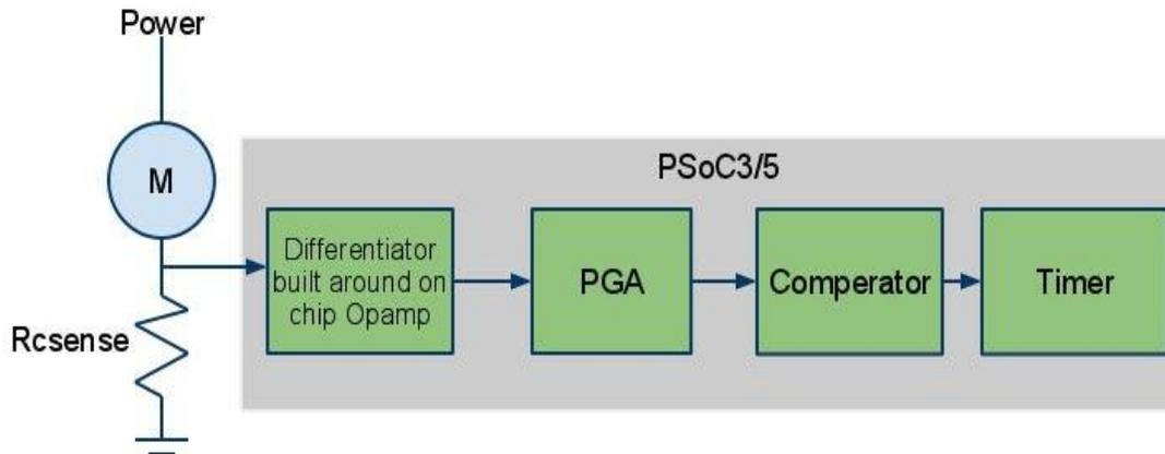
**Figure 3: Measuring commutation frequency**
