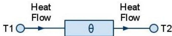
Figure1: Thermal equivalent circuit
