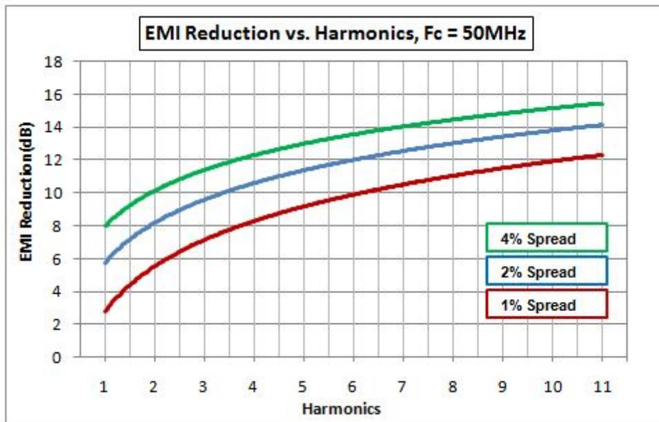
Figure 4: EMI reduction vs. Harmonics
