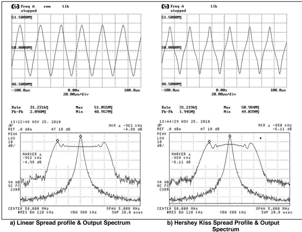
**Figure 5: Comparison between Triangular and Hershey Kiss Spread profiles**
