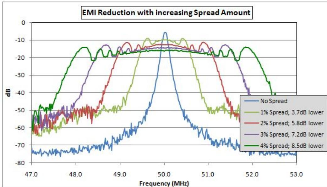
Figure 3: EMI reduction with Increasing Spread amount
