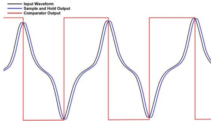
Figure 2: Comparator-based peak detection
