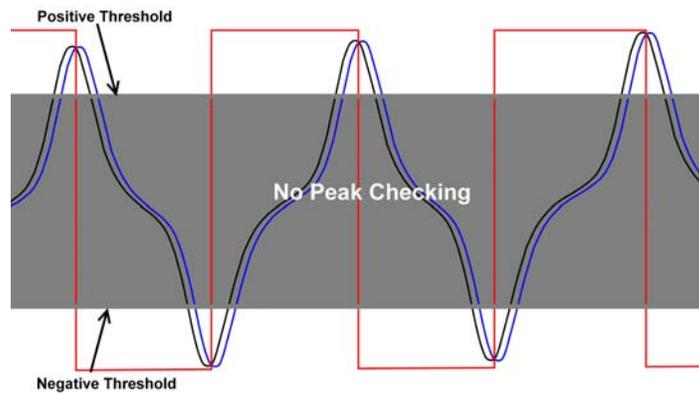
Figure 4: Windowed comparator
