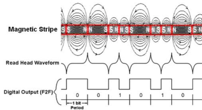
Figure 1: Magnetic card waveform
