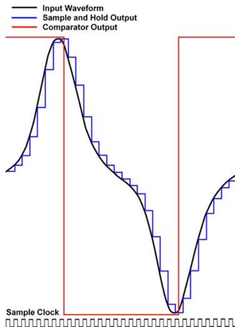
Figure 3: Sample-and-hold peak detection
