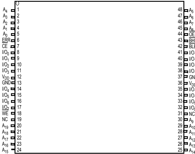
Figure 7. 48-pin TSOP I (12 × 18.4 × 1 mm) Pinout, Single Chip Enable with ERR, CY7C1061GE [6, 7] Package/Grade ID: ZXI
