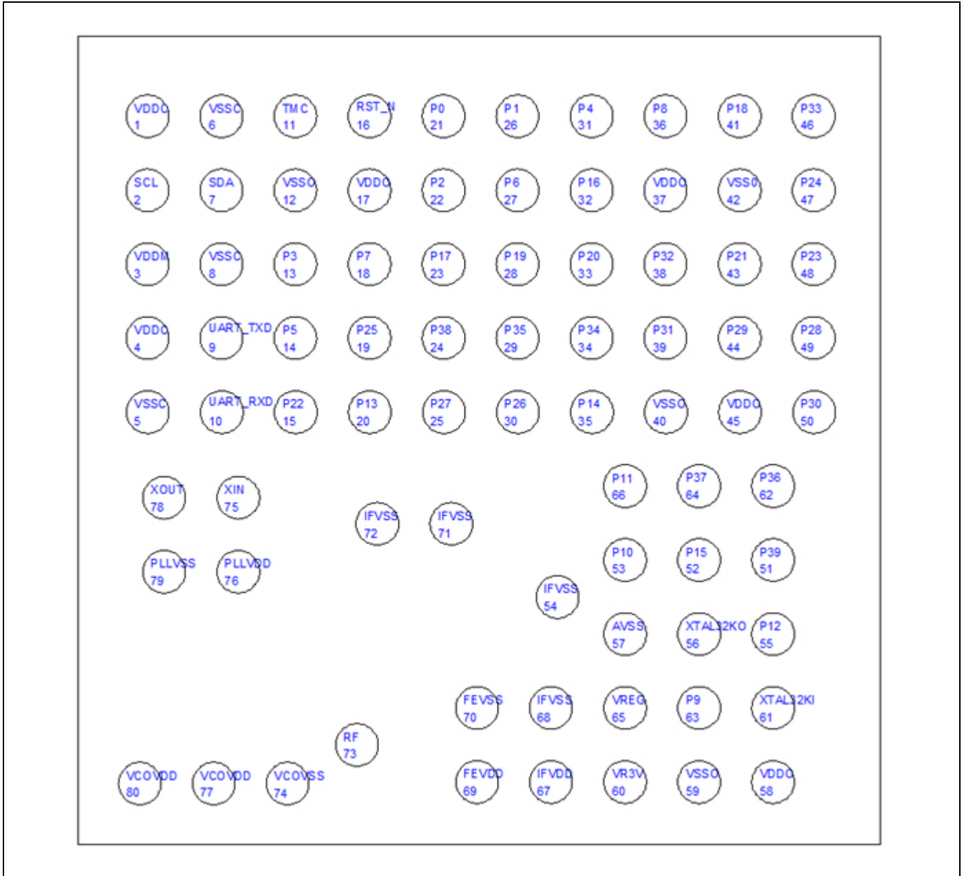
Figure 10. 80-Pin WLCSP Bump Map—Top View of Package with Bumps Facing Down
