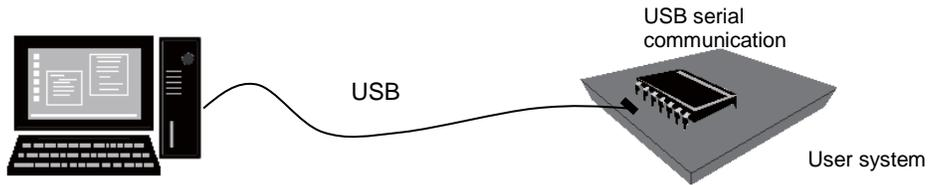
Table 4-3. System Configuration of USB DIRECT Programmer
