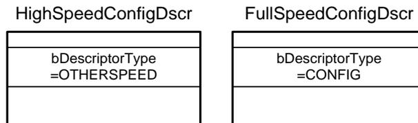
Following a USB bus RESET, the device reverts to FS operation. Therefore, in the USB Reset Interrupt Service Routine, the firmware marks the descriptors ([Figure 3](#)). It also sets pointers to each descriptor (*pConfigDscr* and *pOtherConfigDscr*) for use during enumeration. If the device is plugged into a full-speed port, this designation remains.
